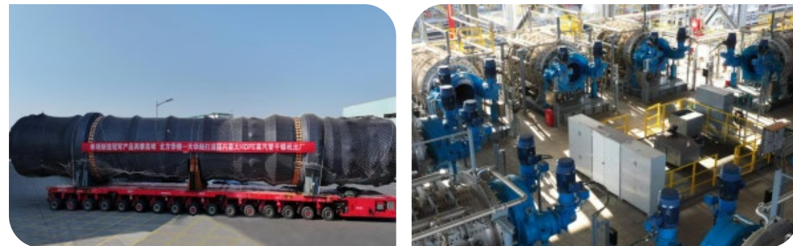
China's largest High-Density Polyethylene (HDPE) steam tube dryer
